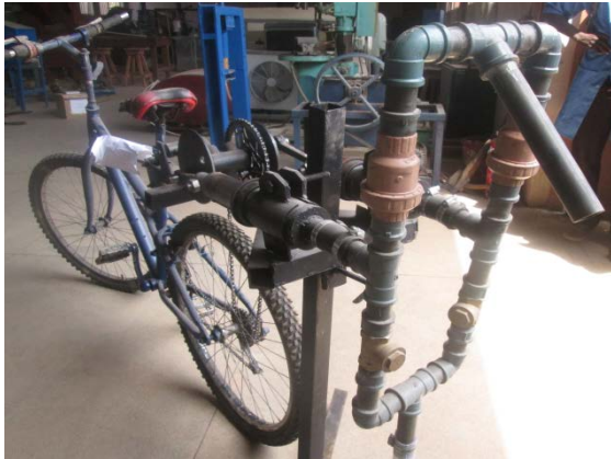
Fig.4: Pedal Powered water pump Machine developed
